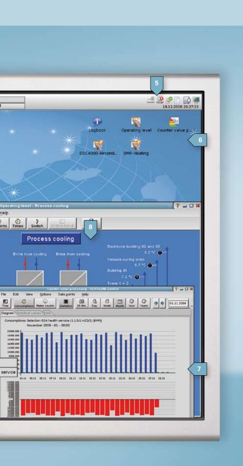
A comprehensive system monitor constantly provides information on the status of the system. It shows information about hardware components being deployed, about network utilization, hard disk activity and available memory.
